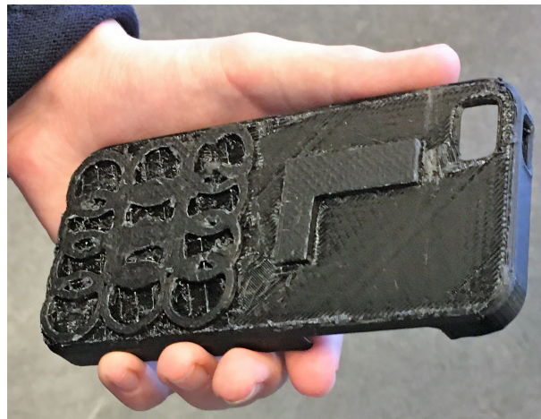
Figure 3.10: Design fails because of support, after this the pupils refrained from using support for future covers.
