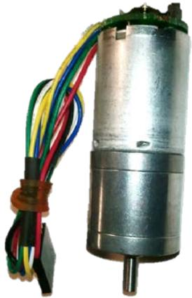
172:1 geared motor with 48 CPR Encoder mounted with a press-fit sleeve around the gear box and set screws attaching it to the frame
