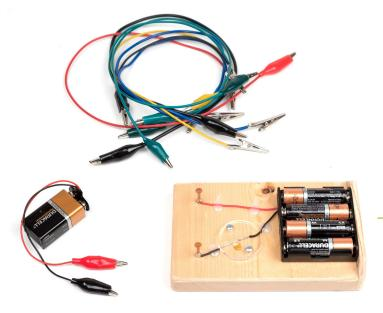
Power supplies and alligator clip leads are important to power the light sources and/or slow motors. We offer both 9-volt and AA power supplies mounted on wood blocks. These power supplies are the same ones we use for the Circuit Boards activity.
