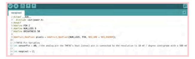
In the variable section, we defined the output pin for the LEDs (2), the number of LEDs (10), the brightness (50), the input pin for the sensor (A0) and called the libraries.
