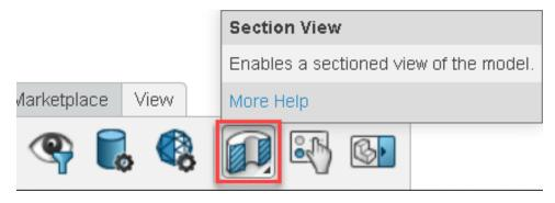
18. [1] Select the different default planes until you find the one that sections the model parallel to the numbered face you oriented on the bottom. If necessary, [2] use the "Flip direction" toggle to create a section view similar to this:
