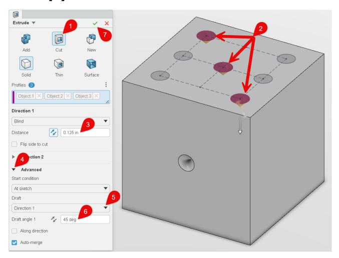
33. Repeat steps 27 through 32 four more times to paste the circle sketch onto the remaining faces of the die and create cuts for the dots. Each time, select a different quantity and position of circles to create the classic 1 through 7 numbered dot patterns.
