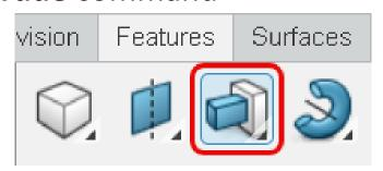
32. [1] Click **Cut**, [2] select the three circles shown below, [3] Set the extrude distance to **0.125 in**, [4] expand the Advanced section, [5] turn on draft in **Direction 1**, [6] set the draft angle to **45 deg**, and then [7] click **OK**
