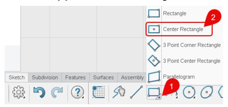
8. [1] Click the origin to place the center of the rectangle, then move your cursor up and to the right to roughly size the rectangle, finally [2] click to place the upper right-hand corner of the rectangle
