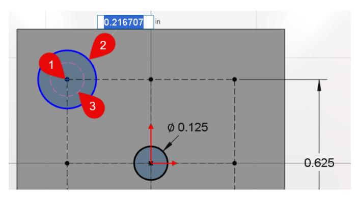
NOTE: snapping to the pink, dashed circle creates an equal constraint to the diameter of the first circle.
