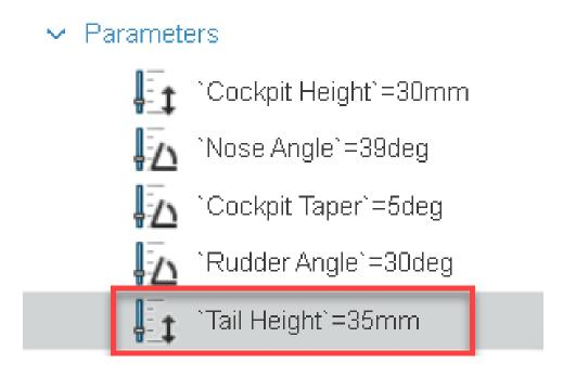
14. This parameter has an unlimited value range. [1] Enter any number into the "Value" field (it should still be small enough to fit on a piece of balsa), [2] Click "Apply" to update the model, [3] Click the OK checkmark to close the dialog
