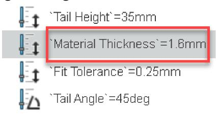
17. [1] Enter the thickness of the wood in the "Value" field, [2] Press "Apply" to update the model, [3] Click the OK checkmark to close the dialog
