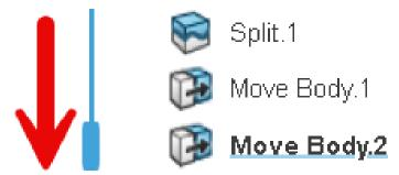
\*\*\*NOTE: This will spread the two halves of the mold apart. Technically this is not where we want to add our inserted geometry, but it will make it easier to see and select it, so we'll proceed this way for now and deal with reordering things later)
