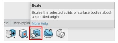
16. [1] Select the inserted spinning top body, [2] type a scale factor of 1.5, [3] Click OK
