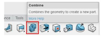
18. [1] Click the "Subtract" button, [2] Select the left half of the mold, [3] Select the right half of the mold, [4] Click in the "Tool bodies" selection box to give it focus (it will turn blue to let you know that your next selection will go into there), [5] Select the inserted spinning top body, [6] Click OK
