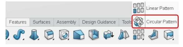
14. [1] Select a face of the extruded decoration you just created, [2] click in the "Pattern Axis" selection box to give it focus, [3] select the circular edge of the hole at the center of the pinwheel, [4] change the "Number of instances" to match the number of blades on your pinwheel, then [5] click OK
